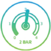
When the radiators are hot this is normal pressure
